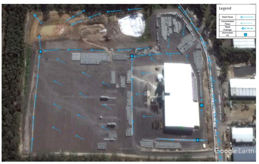
Figure - Overland Drainage Path Diagram
