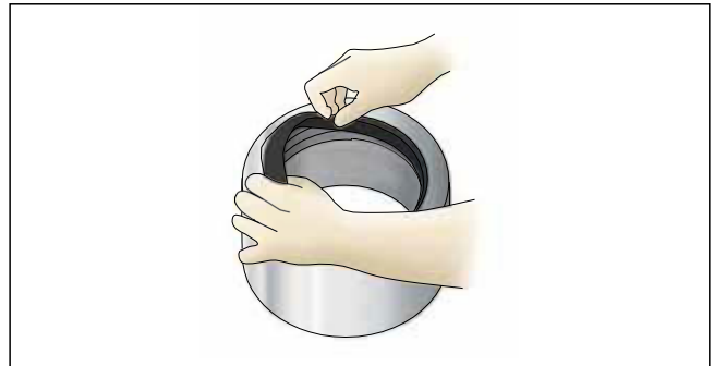
Figure 27 - SuperTite Coupling Installation
